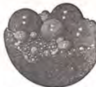
ROLL ON: This theoretical model has ball bearings arranged so that none slips against another.
